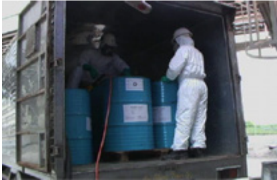
Emptying PCB drums for trial burn
