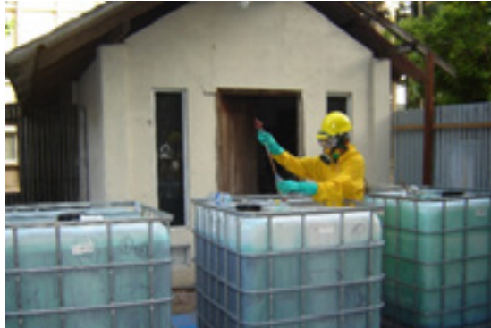
Trial burn of PCBs -Pyralene oil with 56-62% of PCB's, 33-38% tri-chloro-benzene, 5-6% tetra-chloro-benzene
