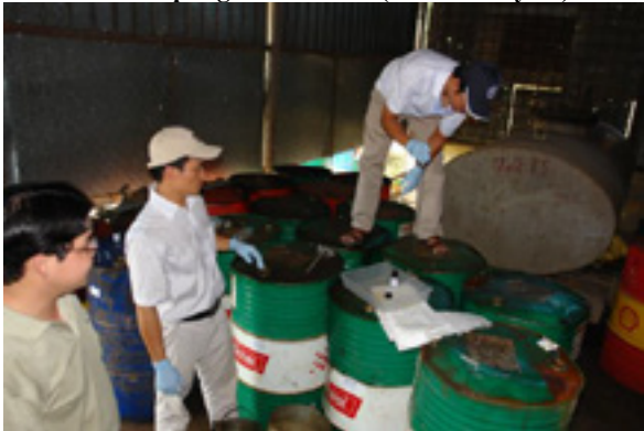
Picture 25: Sampling of oil drums (different layers)
