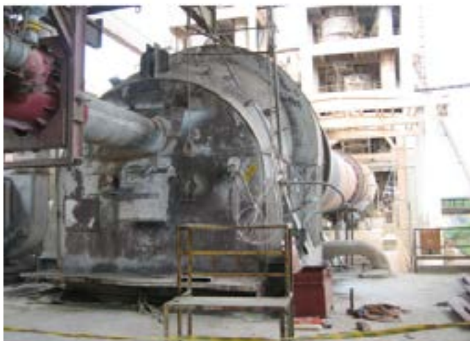
Trial burn of PCBs -Pyralene oil with 56-62% of PCB's, 33-38% tri-chloro-benzene, 5-6% tetra-chloro-benzene
