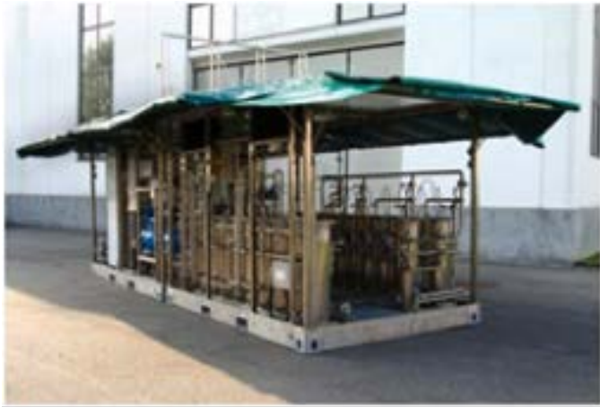
CDP Process ® and DMU- Containerized unit connected with shunt reactor (500 kV) on-load treatment (Brasil 2010)
