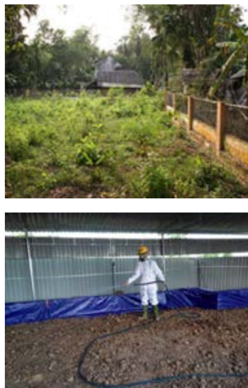
Figure 4. Left a remediated site, with containment of POP residues in the soil, restricted site-use and, monitoring and aftercare and right preparation of anoxic phase of the soil remediation Pilot to test bio-degradation of POP pesticides in soil using Daramend 3 .
