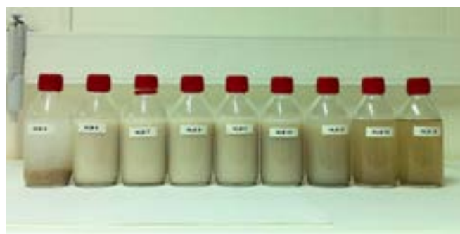
Figure 2. Determination of the required HLB for HCH DNAPL
