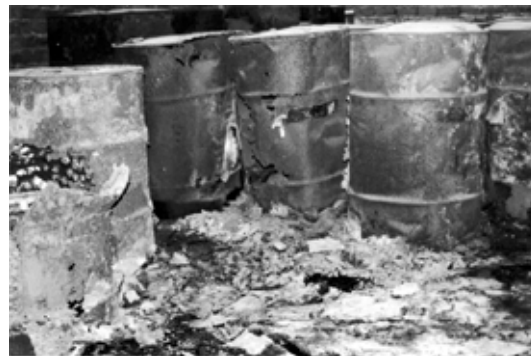
Yet another example of severely deteriorated pesticide stocks in Tete Province, Mozambique. Most of these drums physically disintegrated when man-handled.
