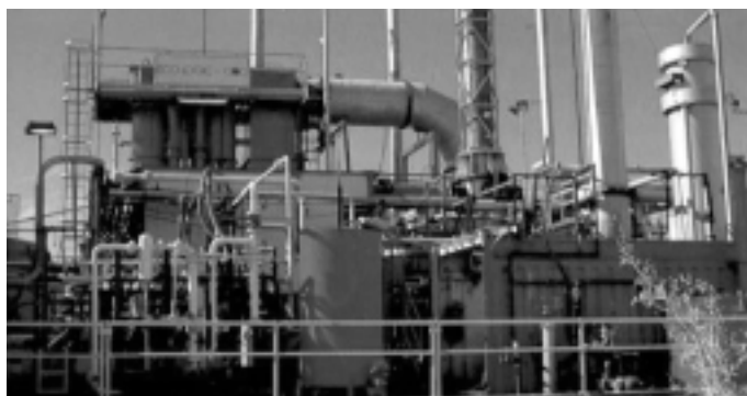
Eco Logic's Full-Scale GPCR Reactor and Scrubbing System in Kwinana, Western Australia
