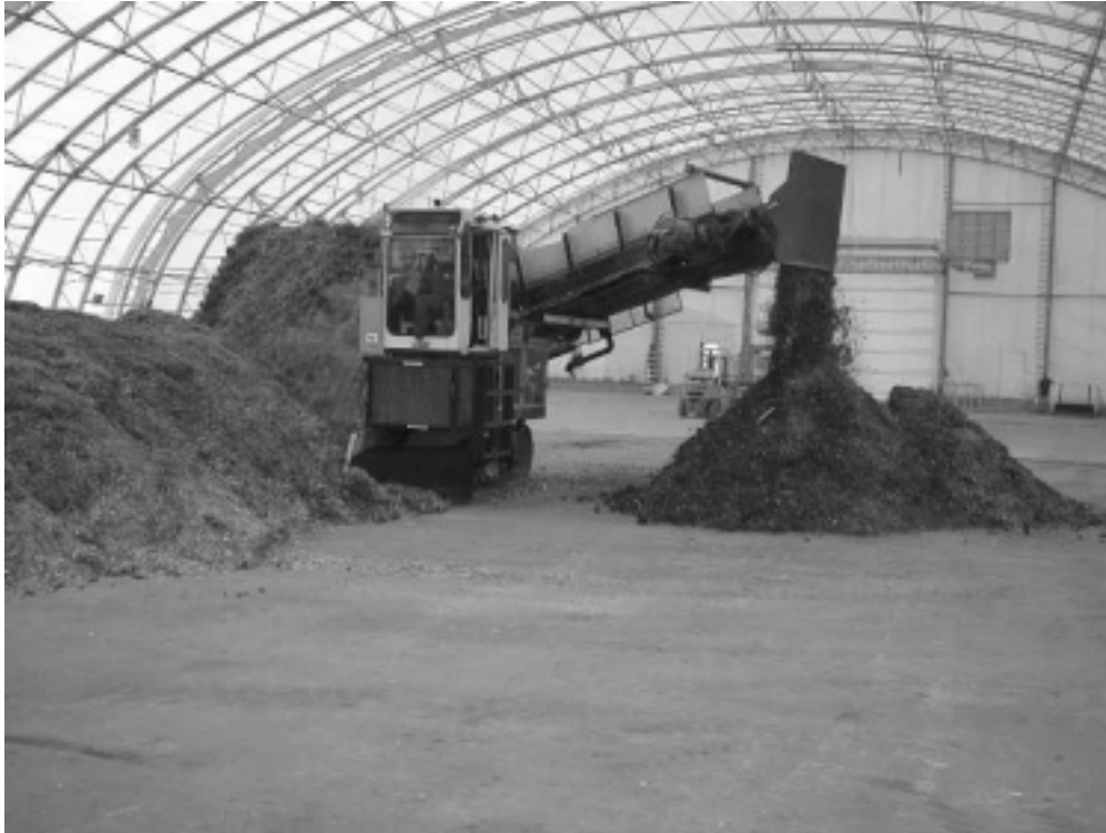
Figure 1. The windrow turner SCAT 4932 being used to mix amendments
