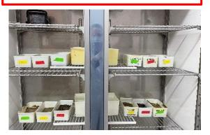
Temperature:26°C Humidity (60% of soil water holding capacity) % Degradation of 1,2,4-TCB,  $\alpha$ -HCH,  $\beta$ -HCH  $\Longrightarrow$  GC/MS
