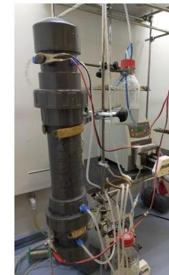
To evaluate how interact the different processes that are induced when electric fields are applied to aged silt from the Sardas landfill (Sabiñánigo, Huesca).
