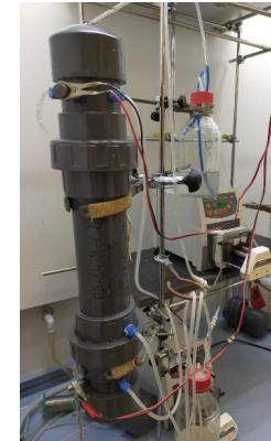
To evaluate the viability of electrokinetic remediation for the treatment of aged silt from the Sardas landfill (Sabiñánigo, Huesca).
